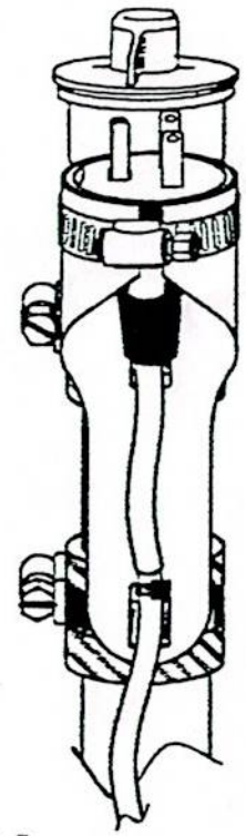
FIG. 5 HARNESS PLUG INSTALLED IN PMT SECURED WITH WORM CLAMP AND TIEWRAP. BE SURE PLUG IS ACCESSIBLE THROUGH OIL DOOR.
