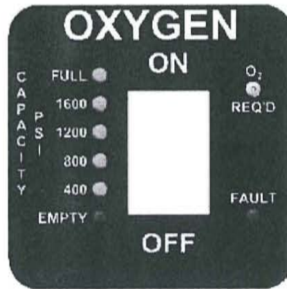
Figure 2 – Oxygen Control Panel
