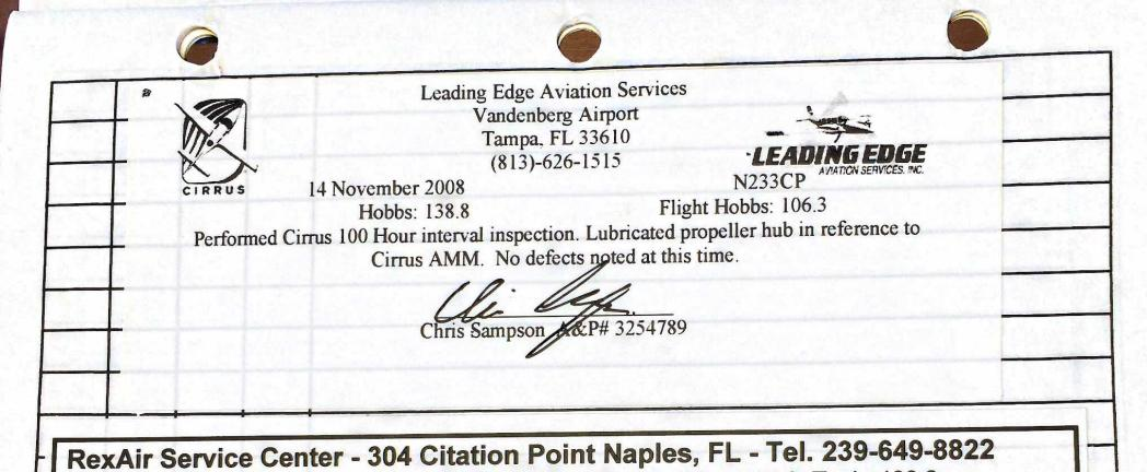
10-01-2009 N233CP Cirrus SR-22 G3 Turbo S/N 3150 Hobbs: 267.0 Tach: 199.8 Hartzell Model: PHC-J3YF-IN s/n: FP6919B TTSN: 199.8 Maintenance: Propeller Annual WO# 2009 Performed 100Hr inspection IAW Cirrus SR-22 maintenance manual and FAR 43 App (D). I certify that this propeller has been inspected IAW an annual inspection and is determined to be in airworthy condition at this time.-END- David M. Montgomery A.&P. 159423106 I.A.
